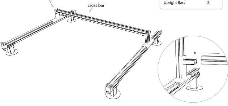
Install (1) upright bar into each upright bracket. Hand-tighten the allen bolts on the upright brackets.
