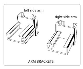
NOTE: You will have left and right sided arm brackets. When installed on the rack, the eye bolts will be towards the inside of the rack.
