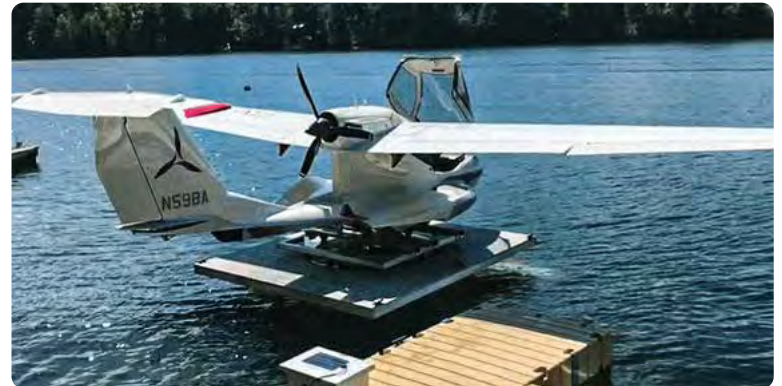
Above: Seaplane lift utilizing a stock hydraulic lift with a custom turntable platform.
