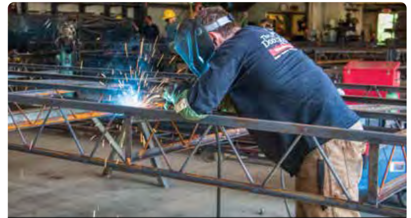
Dock frames being manufactured in our Vermont Facility
