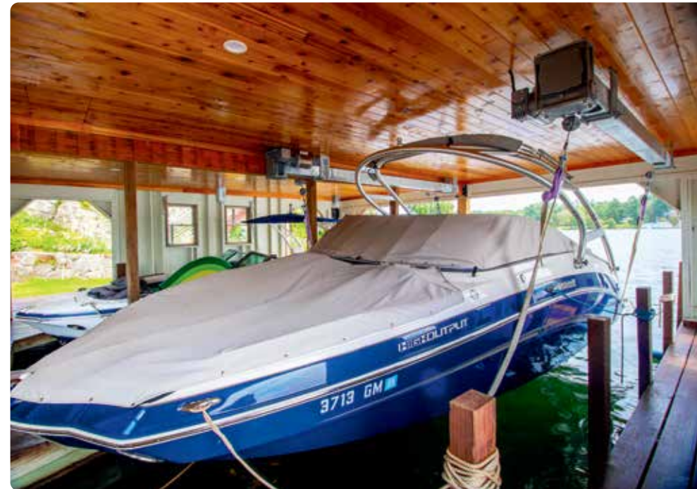
Above: Sling style system for shallow water applications.
