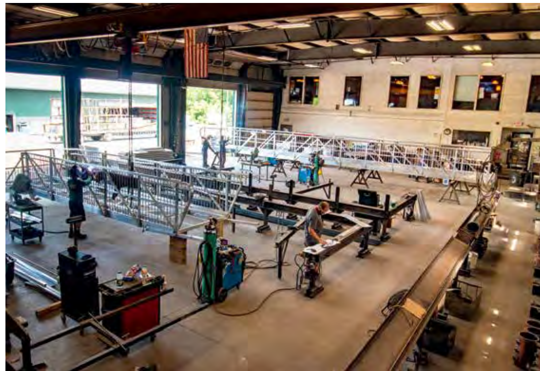
Above: 6' x 48' aluminum gangway to steel truss floating dock designed for a high freeboard marine research vessel. Below Left: ADA access boarding gangway with spindle rail. Below Right: Both gangways during fabrication in our workshop.
