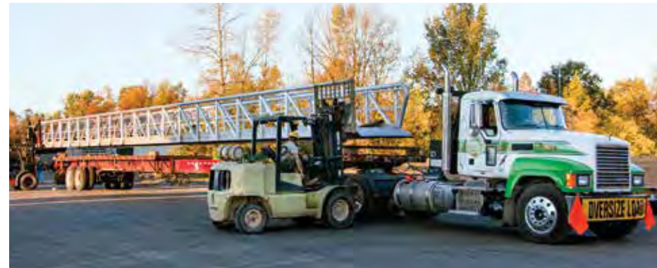
80' long gangway being loaded for delivery.
